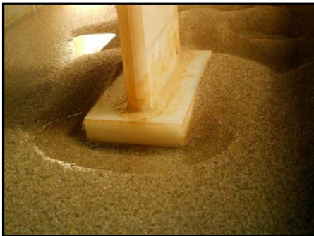
Fig. 9. Observed scour depth at complex pier before undercutting the pile cap
